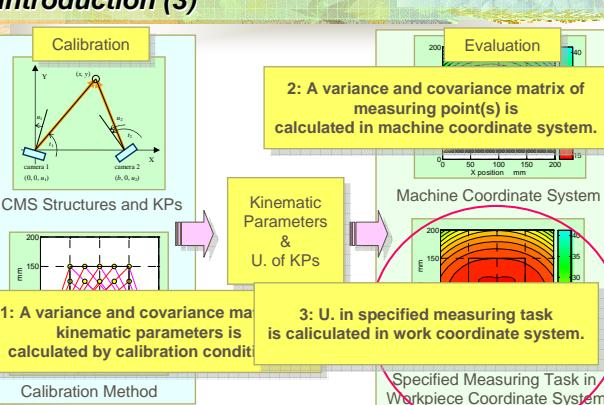
1: A variance and covariance matrix of kinematic parameters is calculated by calibration condition.
