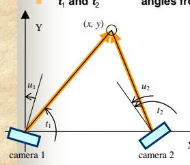
$$\begin{aligned} \begin{pmatrix} x \\ y \end{pmatrix} &= \mathbf{f}(\mathbf{p}, \mathbf{q}) = \begin{pmatrix} \frac{b \tan(t_2 - u_2)}{\tan(t_2 - u_2) - \tan(t_1 - u_1)} \\ \frac{b \tan(t_1 - u_1) \tan(t_2 - u_2)}{\tan(t_2 - u_2) - \tan(t_1 - u_1)} \end{pmatrix} \\ \mathbf{p} &= \begin{pmatrix} u_1 \\ u_2 \\ b \end{pmatrix}, \quad \mathbf{q} = \begin{pmatrix} t_1 \\ t_2 \end{pmatrix} \end{aligned} \quad \text{Equation (7)}$$
