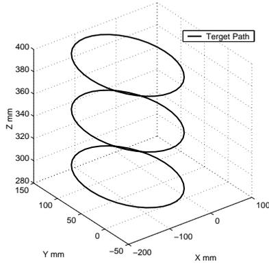
Fig. 2 Measuring circles (target paths) for calibration of parallel mechanism
