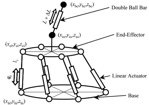
Fig. 1 Kinematic model for calibration of parallel mechanism
