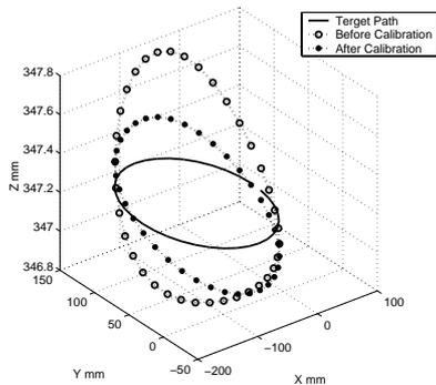
Fig. 3 Positioning errors before and after calibration on target path
