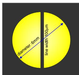
FIGURE 4: A pattern with a rectangular masking, with which a discoidal cured resin with a submicron groove should be fabricated.
