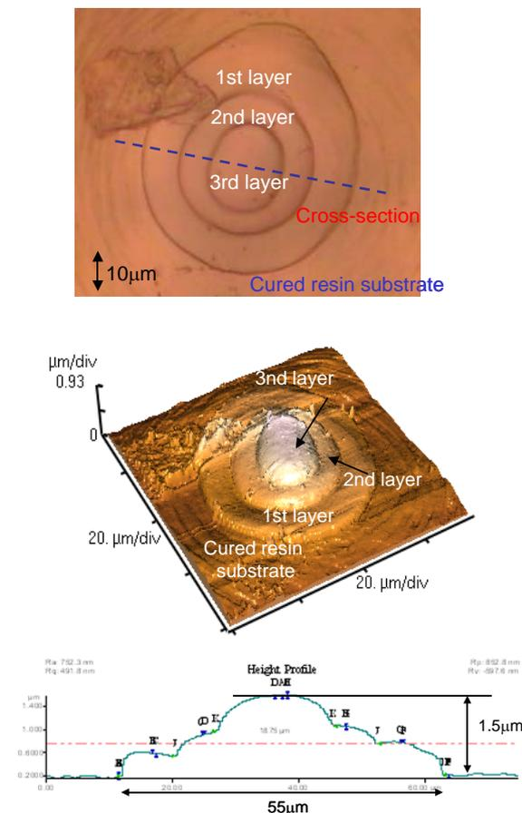
FIGURE 7: Fabricated nano-steps. (TOP) Microscope image. (Middle) AFM image. (Bottom) Cross section of the AFM.
