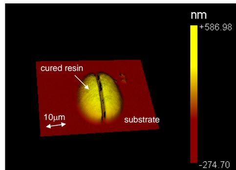
FIGURE 5: The result of the fabricated pattern analyzed by a white light interferometer, which suggests the possibility of 2D submicron fabrication.
