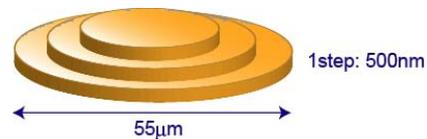
FIGURE 6: These steps are attempted to fabricate to verify the lamination process.
