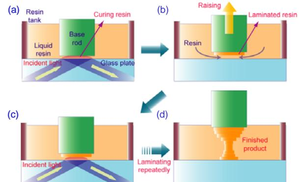
FIGURE 2: Schematic diagram of the nano-stereolithography method using evanescent light.
