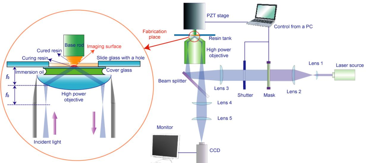
FIGURE 3: A developed nano-stereolithography system using evanescent light (Right) A modulated beam passes through the periphery of the objective's pupils and evanescent light is generated in the liquid resin. (Left) The exposure surface is equivalent of the imaging surface of the variable mask.
