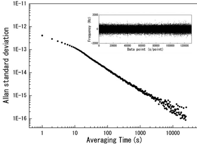
Fig. 3. Frequency differences between two combs (inset) and corresponding Allan deviation.
