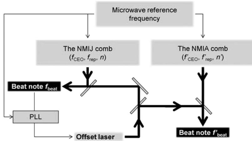
Fig. 2. Diagram of the measurement capability validation of combs. An offset laser is locked to the NMIJ comb and measured with the NMIA comb. The beat frequencies between the offset laser and each comb are simultaneously counted.
