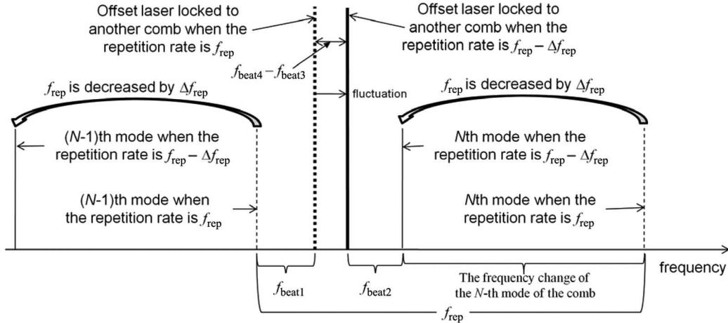
Fig. 4. Frequency relations between the comb mode and the measured laser in mode-number determination.
