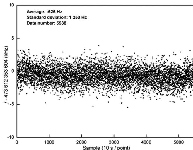
Fig. 1. Measurement results of the HeNe/I<sub>2</sub> laser N1 using a fiber comb.
