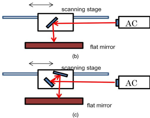
Fig. 4 Experimental set up for profile measurement:
