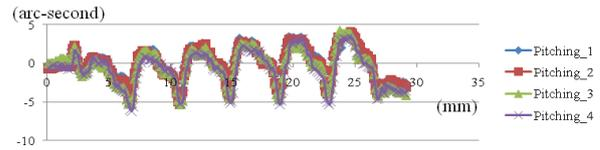
Fig. 5 Pitching error of scanning stage
