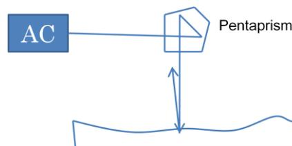
Fig.1 Principle of scanning deflectometry method with pentagon prism
