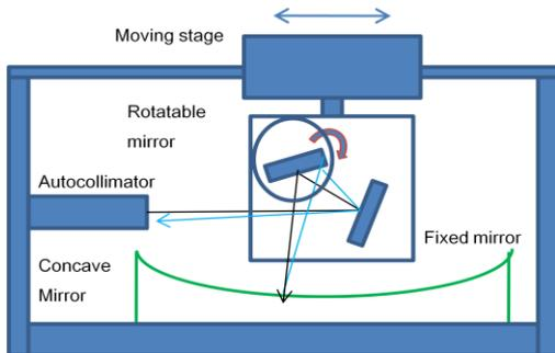
Fig.2 Principle of scanning deflectometry method with rotatable mirror
