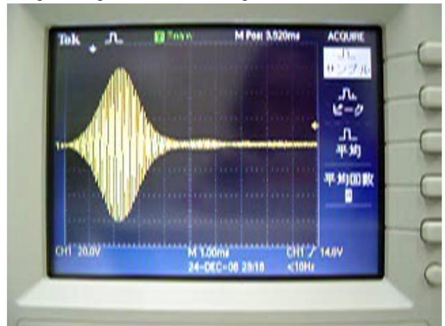
Fig. 8: Observed constructive interference when the two pairs of pulse trains were overlapped.
