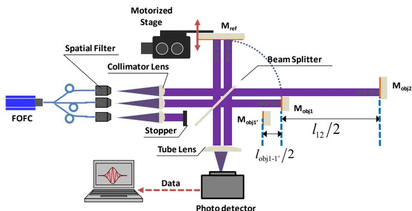
Fig 1. Optical schematic.
