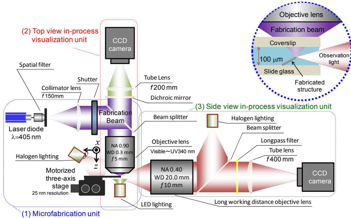
Figure 3: 3-D microstructure fabrication system by photocatalyst nanoparticles.
