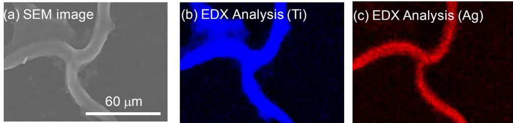
Figure 6: SEM-EDX analysis. (a) SEM image. (b) EDX image of Ti. (c) EDX image of Ag.
