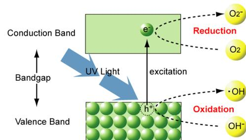
Figure 1: Photocatalytic mechanism.
