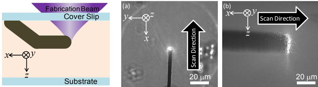
Figure 5: In-process visualization of the proposed microfabrication method. (a) With the top view unit. (b) With the side view unit.
