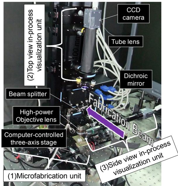
Figure 4: Photograph of developed 3-D microstructure fabrication system.
