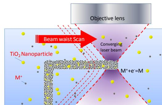
Figure 2: Concept of 3-D microstructure fabrication by photocatalyst nanoparticles.
