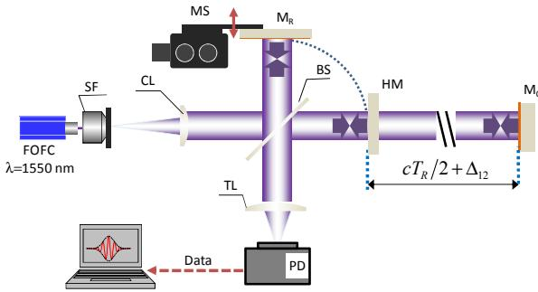
Fig. 2. Optical layout. FOFC: femtosecond optical frequency comb, CL: collimator lens, TL: Tube Lens, BS: beam splitter, PD: photo detector, MS: motorized stage, HM: half mirror,  $M_{R-O}$ : mirrors.
