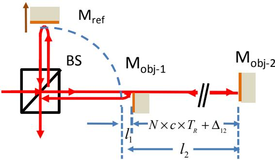
Fig. 1. Multiple-pulse train interference for length measurement.
