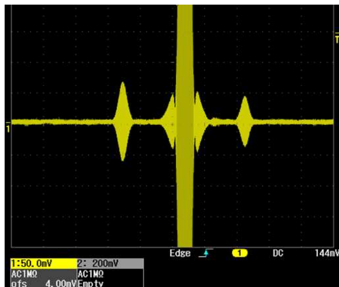
Fig. 3 Interference fringes with different relative delays between two beams
