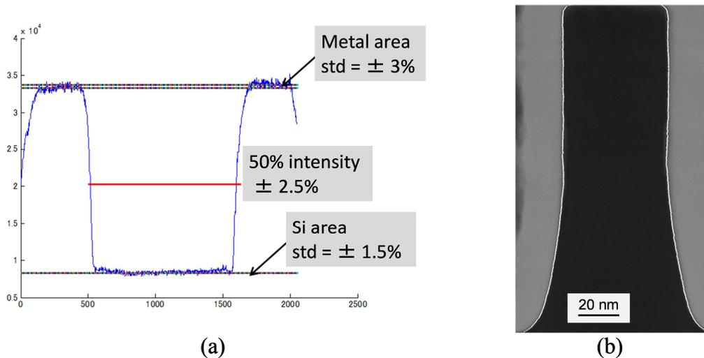
Figure 3. Definition of the edge as the SiO<sub>2</sub>-Air interface; (a) intensity graph of the STEM dark field image, and (b) edge detections from top to bottom.
