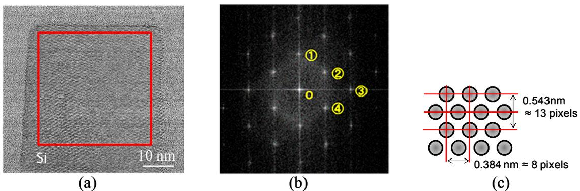
Figure 4. 2D Fourier analysis of STEM image; (a) inside of Si lattice is extracted, (b) transformed to a frequency domain image with zero padding and four main peaks, and (c) Si lattice structure.
