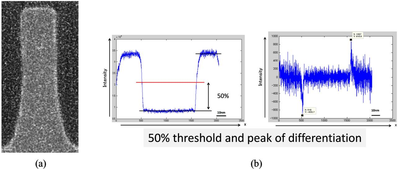
Figure 5. Future works; (a) sectional SEM images, and (b) comparison between the line width by 50% threshold level and peak of differentiation.
