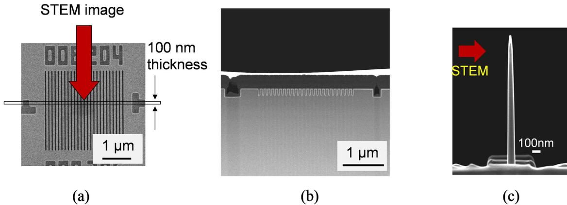
Figure 1. Sample for STEM image; (a) position of a thin specimen of 100 nm thickness by FIB (Focused Ion Beam) micro sampling system in the CD-SEM image, (b) STEM image of standard line width in low magnification, and (c) thin specimen of 100 nm.
