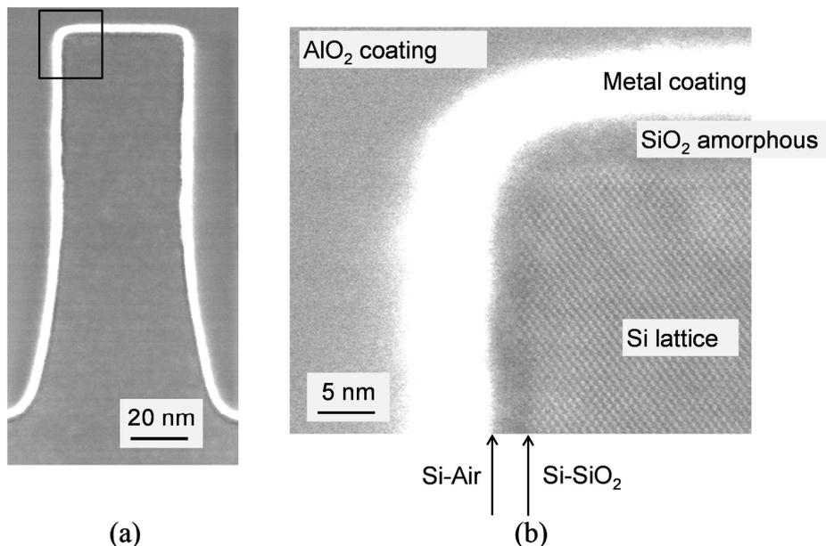
Figure 2. Si lattice structures and two interfaces ( $\text{Si-SiO}_2$  and  $\text{SiO}_2\text{-Air}$ ) are observed by a STEM dark field image of the thin spacemen with metal coating; (a) STEM dark field image, and (b) Si lattice,  $\text{SiO}_2$  amorphous and metal coating in the high magnification image.
