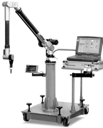
Fig.1 Articulating CMM with six rotational joints and sensors
