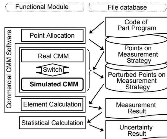
Fig. 1. Scheme of CMM uncertainty evaluation by Monte Carlo simulation
