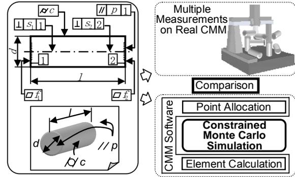
Fig. 5. Comparison between real measurement and CMS result
