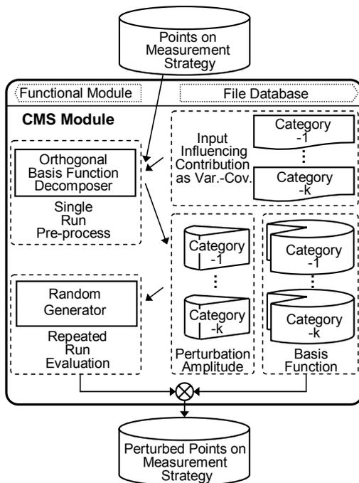
Fig. 2. Scheme of constrained Monte Carlo simulation
