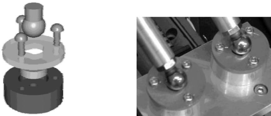
**Fig. 11** Construction and photograph of the magnet ball joints
