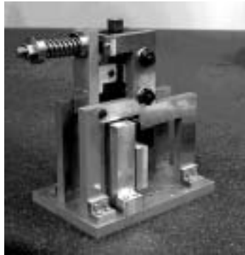
Fig. 8: New Z stage using magnet.
