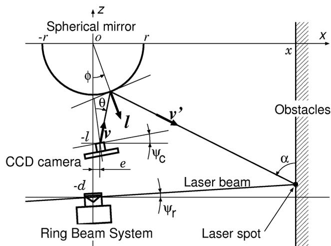
Figure 7. New geometrical model with geometrical errors.
