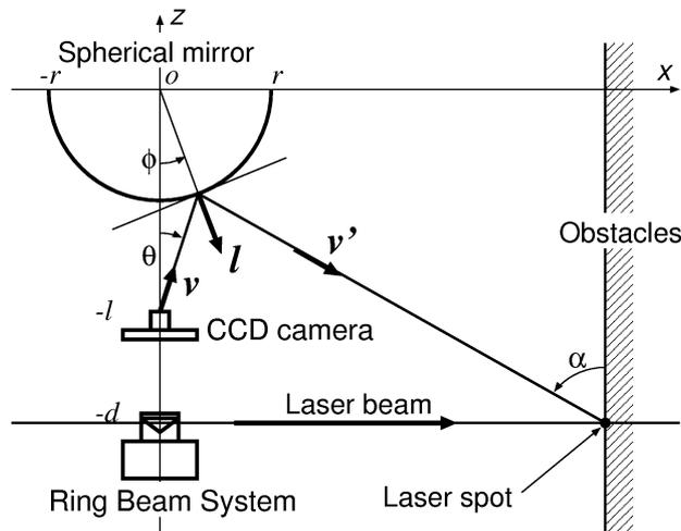
**Figure 1.** Geometric model of obstacle detection system.
