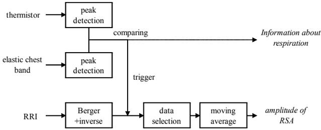
Figure 3: Schematic diagram of the real-time signal processing method for extracting RSA amplitude, which is adoptive under the condition of body motion of the subject.
