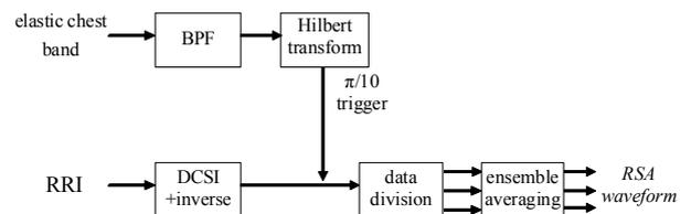
Figure 6: Schematic diagram of the signal processing method for extracting RSA waveform. The BPF box refers to band-pass filtering.
