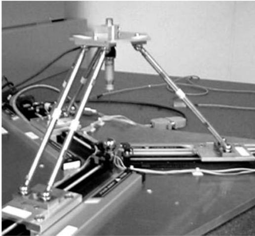
Fig.5 Prototype of Parallel CMM
