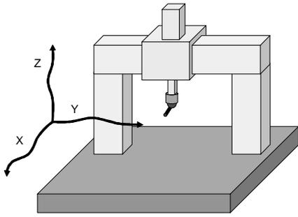
Fig.1 Conventional CMM by Cartesian Coordinate System has 3 Kinematic Parameters and 18 Form-Deviation Parameters
