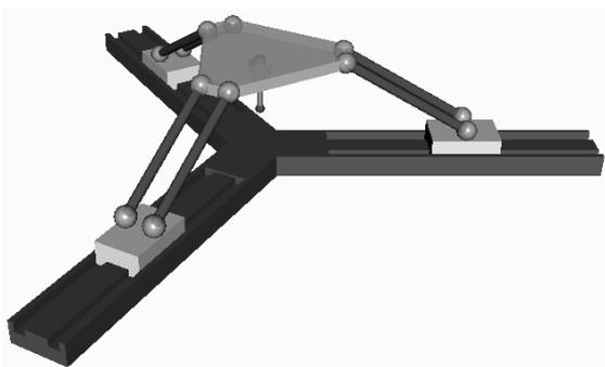
Fig.4 3DOF Parallel Mechanism has 39 Kinematic Parameters
