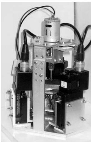
Fig.6 Prototype of Micro Milling Machine
