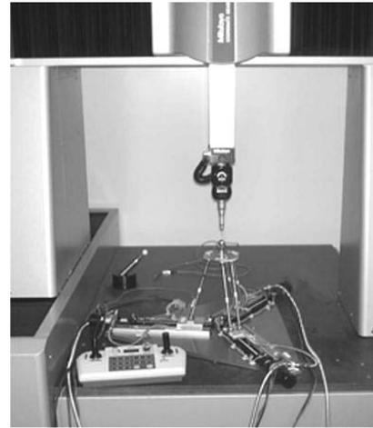
Fig.11 Calibration by Conventional CMM
