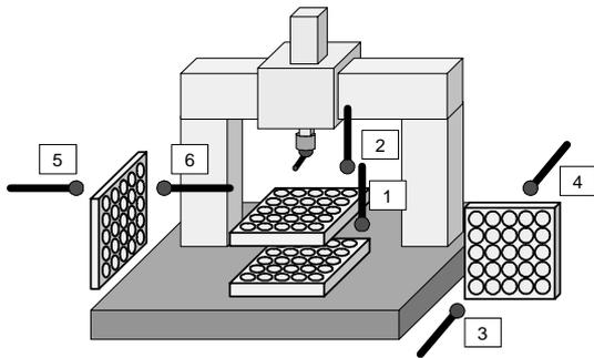
Fig.2 Kinematic and Form-Deviation Calibration Using Ball Plate or Hole Plate
