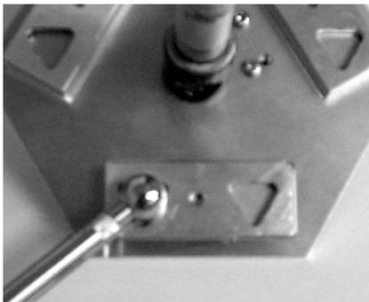
(a) Photograph of Magnetic Spherical Joint
