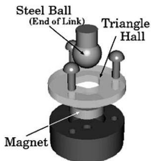
(b) Construction of Magnetic Spherical Joint
