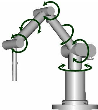
Fig.3 6DOF Articulated Type Robot has 27 Kinematic Parameters
