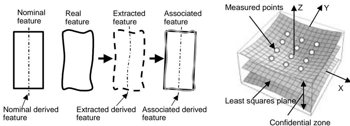
**Figure 1.** Data processing flow in feature-based metrology. **Figure 2.** Confidential zone of measure plane.
