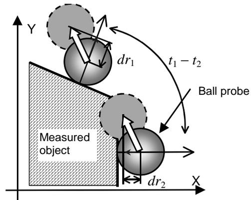
**Figure 6.** Correlation of two measured points by center position errors
