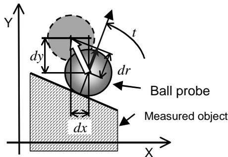
**Figure 7.** Effect of center position errors of ball probe
