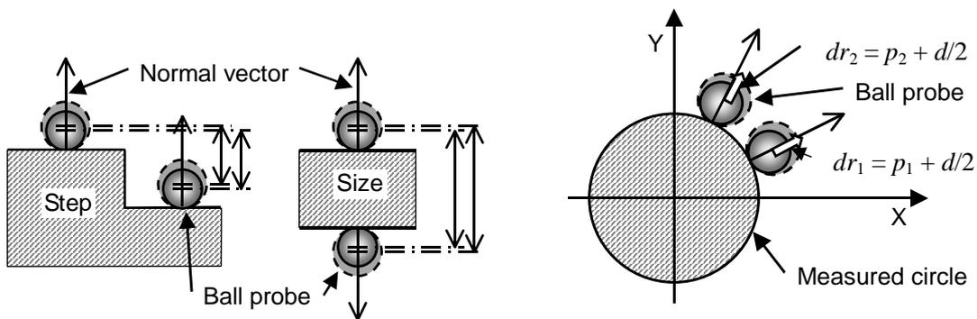
**Figure 5.** Effect of diameter errors of ball probe on **Figure 6.** Correlation of two measured points step dimension and size dimension by effects from diameter error
