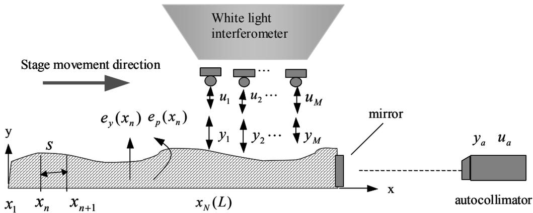
Fig. 2 Scanning system of coupled distance sensors, together with an autocollimator as an additional angle measuring device. A mirror is attached to the moving stage. The autocollimator, the moving stage carrying the sample, and the multi-ball-cantilever is rigidly fixed to the table.
