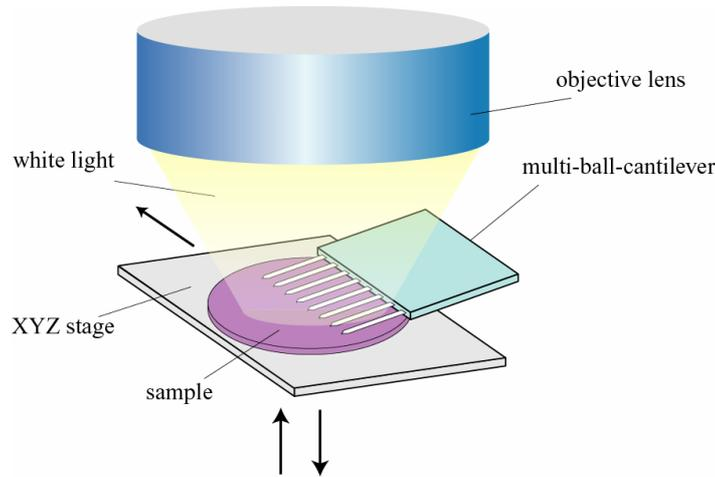
Fig. 1 The multi-ball-cantilever AFM system concept: The multi ball cantilever is fixed, and the sample is moved to contact the cantilevers. The profiles of touched cantilevers are scanned by the white light interferometer.
