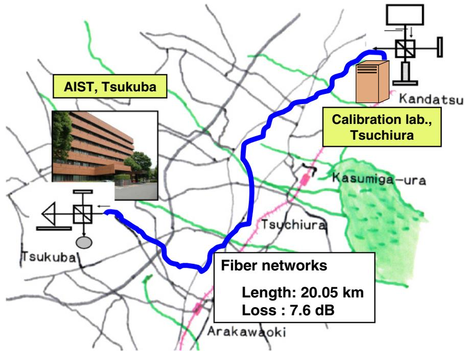
Fig. 1. (Color online) Outline of remote calibration system using optical fiber networks.
