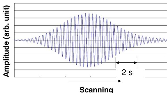
Fig. 5. (Color online) Typical example of low-coherence interference fringes obtained.
