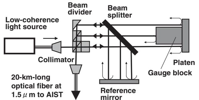
Fig. 3. Setup of the measurement interferometer.
