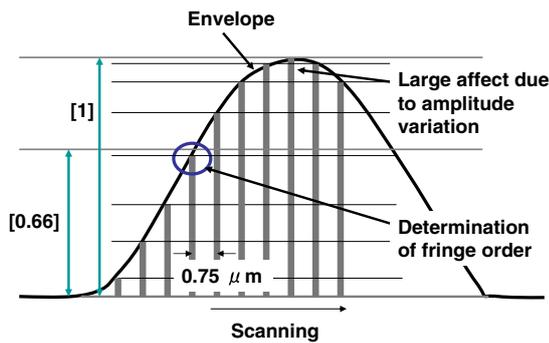
Fig. 2. (Color online) Proposed technique for determining the central fringe order of low-coherence interference fringes obtained.
