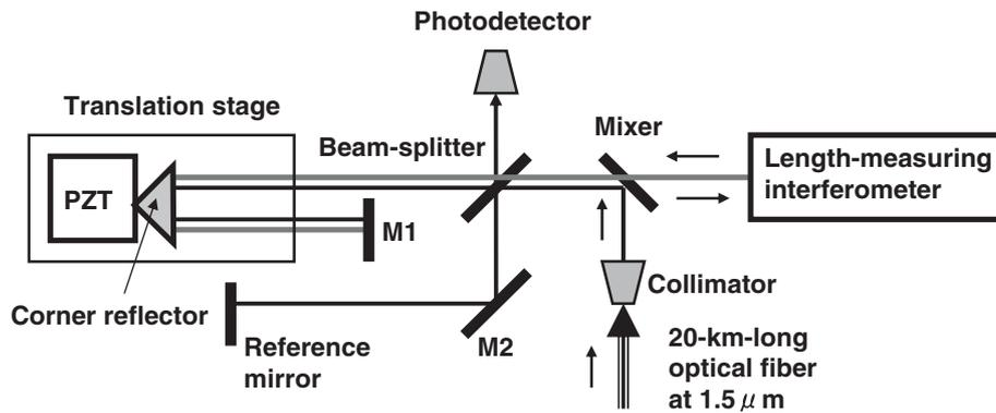
Fig. 4. Setup of the reference interferometer.
