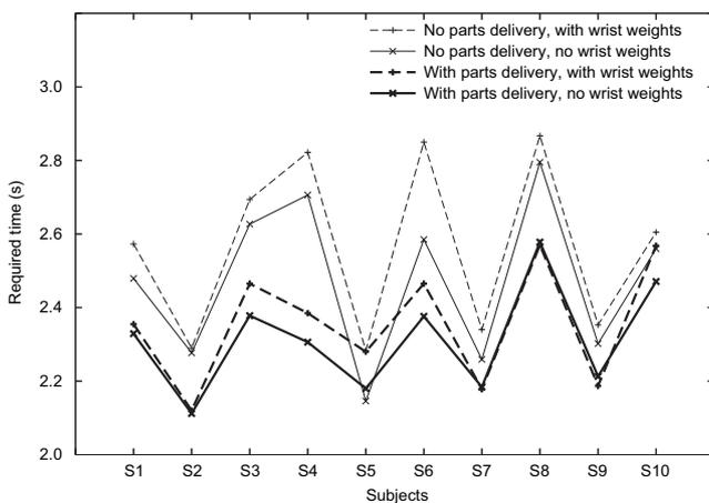
**Fig. 9.** Mean time required for assembly process.
