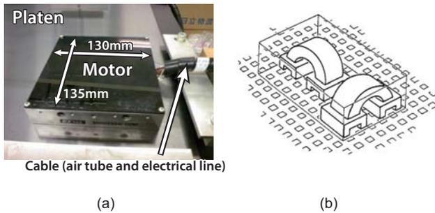
**Fig. 2.** (a) Sawyer-type planar motor and passive iron platen. (b) Mechanism of a Sawyer-type motor.
