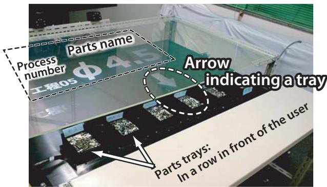
**Fig. 6.** Experimental setup in the case without parts delivery. Assembly information is projected on the desk. Trays in front of the subject do not move.
