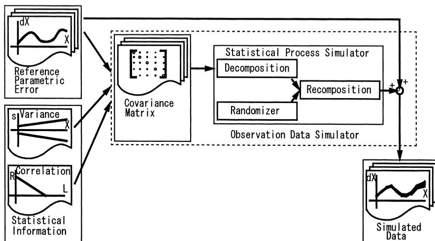
Fig. 2. Schematic of simulation data generation based on decomposition method.
