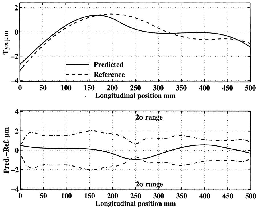
Fig. 6. Example of simulation result by the integrated model, straightness of the X axis.
