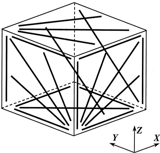
Fig. 4. Measurement strategy adopted for simulation, only by longitudinal displacement.
