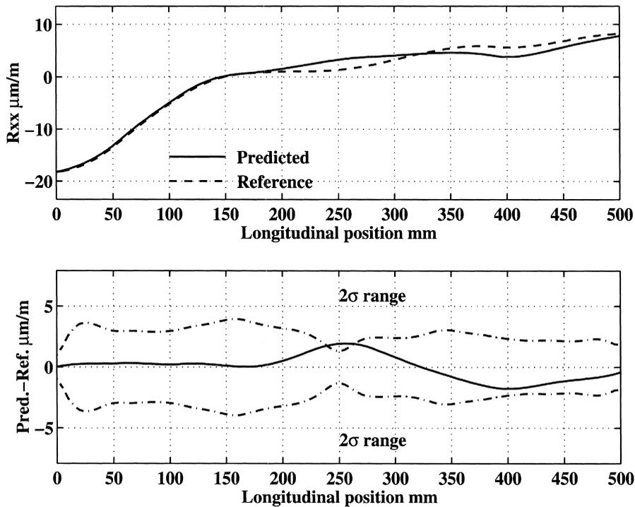
Fig. 7. Example of simulation result by integrated model, roll of the X axis.
