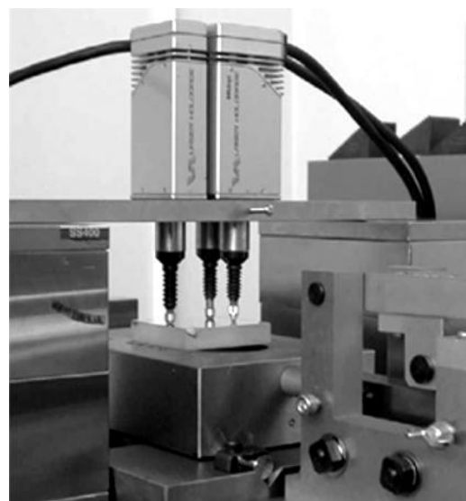
Fig. 8 Photograph of measuring method of tilt angles of X stage
