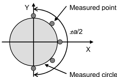
Fig. 4: Measured area  $a$  for partial circle measurement, 5 measured points in  $\pm 90$  deg ( $a = 180$  deg)
