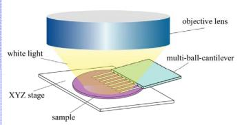
We have proposed a new technique based on AFM theory using mechano-opto-probe.
