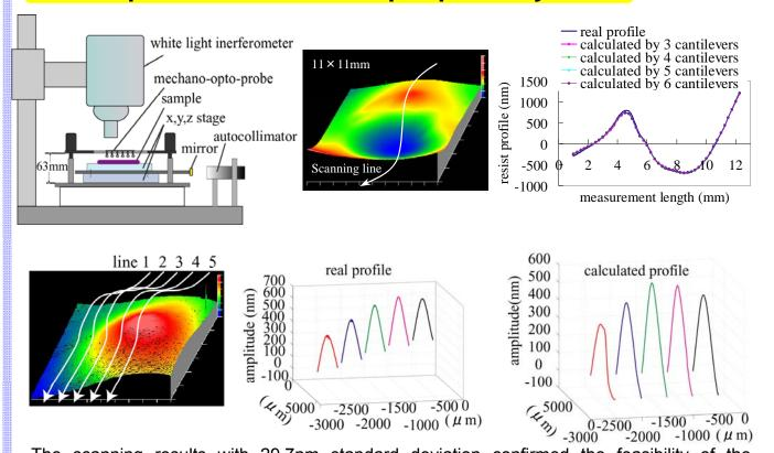
The scanning results with 29.7nm standard deviation confirmed the feasibility of the proposed method in 11.25 mm length resist surface.
